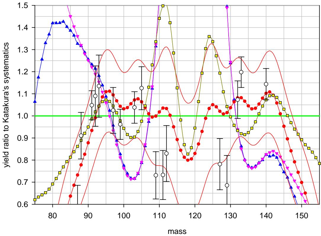
Benchmark A:  $^{239}\text{Pu}$  at 7.9 MeV, post neutron emission yield ratio to Katakura's systematics
